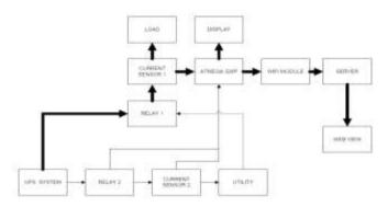
In this case the load is below 70W, at this instant the UPS power the load. Such that the connection from the utility is switched off by relay 1. Here LCD display shows the power drawn by the load. Here the generated power is completely utilized by the load. The current sensor senses the current and the power is calculated .The controller keeps on checking the output of current sensor.
