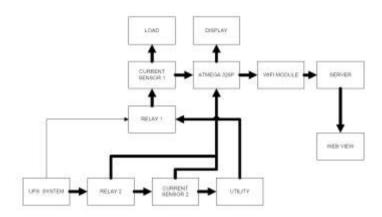
At this instant the load is greater than 70W. Here the relay 1 operates and the utility powers the load. The current sensor reads the current and the power is calculated. Here the display shows the power drawn from the utility. At the same time the relay2 operates to give power to the utility. Here the energy produced by the UPS system at the instant is transferred to the utility system. Thus a transfer of energy from the UPS to the utility occurs.
