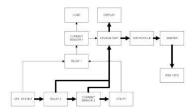
In this case the load is zero. Here the relay 2 operates and gives the power to the utility. To maximize the efficiency of the system, energy produced by the UPS system at the instant is transferred to the utility system. The current sensor senses the current and display shows the power given to the utility.
